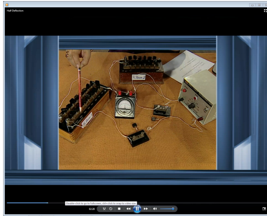
Galvanometer by half deflection method is shown in Fig
